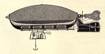
Screw propellers rotate in cylindical casings situated in the girder, and a fan, which is mounted on a universal joint at the stern of the balloon, directs a current of air against an adjacent surface.
